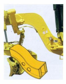
**Circle drive slip clutch** – protects circle shoes and teeth from damage. Should a large rotational force be placed against the blade (as when striking a buried rock) the clutch will slip and the impact load placed against frame will also be absorbed.
