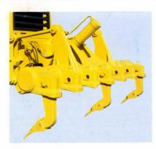
**Rear-mounted ripper:** Four, parallel linkage type. With hydraulically controlled raise and lower functions, this ripper can be used to dig out rocks or hard ground not removable by a scarifier.
