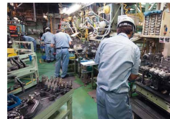
Assembly workshop for control valves, which send oil to hydraulic components
