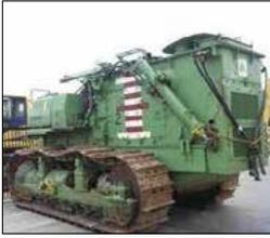
The amphibious bulldozer sent back to the Osaka Plant sustained extensive damage from rust and corrosion.
