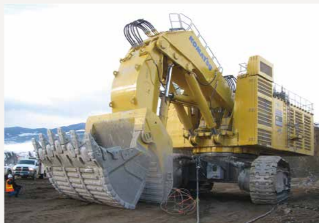
Komatsu PC8000 hydraulic excavator installed with a cast lip and Hensley's three-piece TS1222 system
