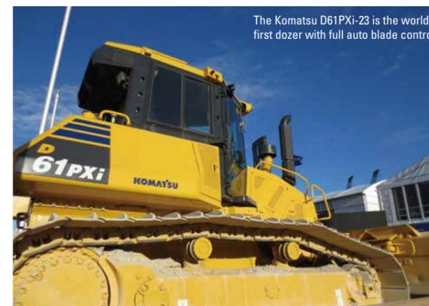
The Komatsu D61PXi-23 is the world's first dozer with full auto blade control.
