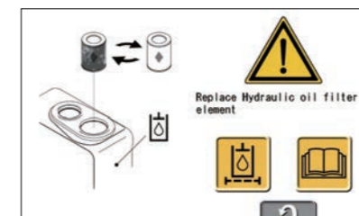
Clogging hydraulic oil filter caution
