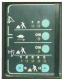
Track shoe slip control panel
