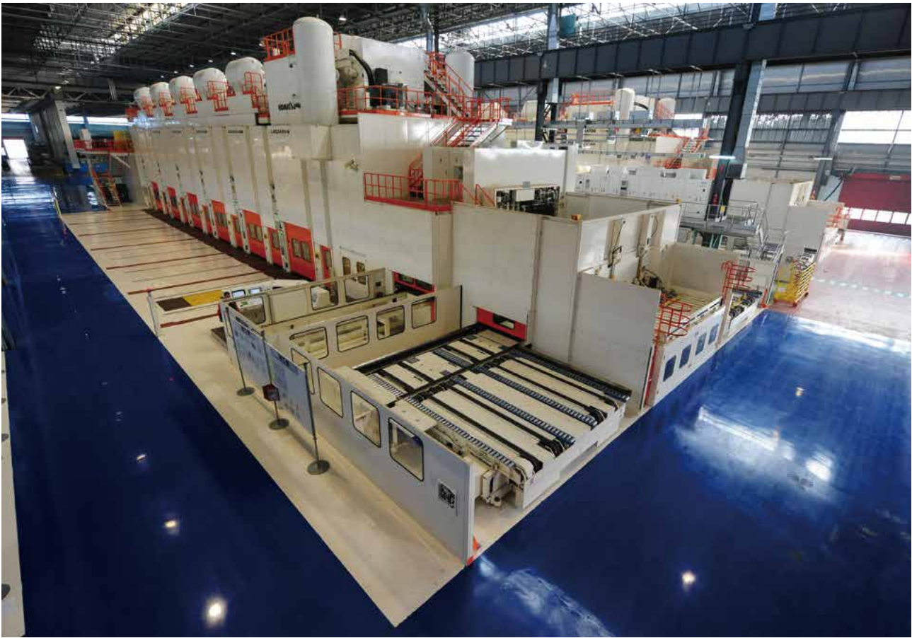
Large press line for machining automobile body panels
