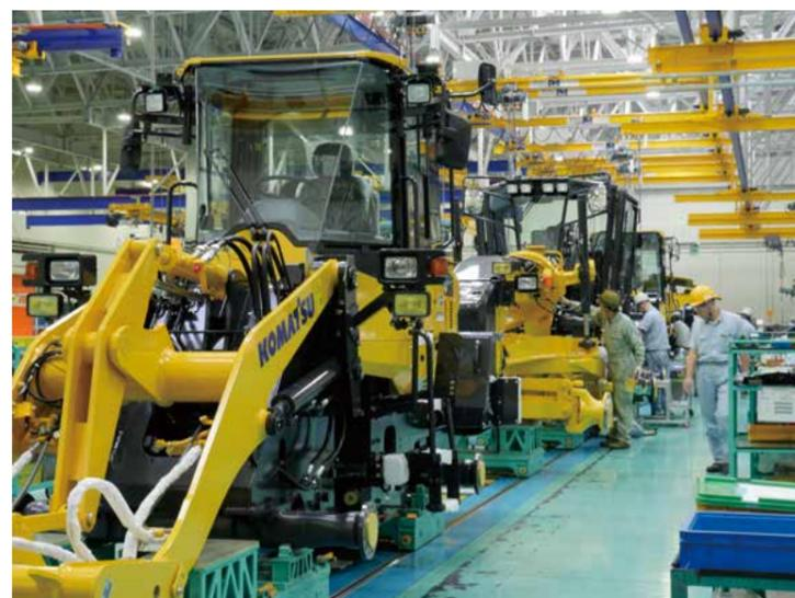
Efficient assembly on the mixed production line for wheel loaders and motor graders
