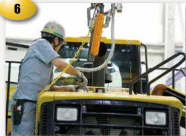
Equipment is supplied with fuel and hydraulic oil. The types and amounts of fuel differ by equipment model and option orders by customers. By scanning a bar code, the hose for the particular type of fuel automatically descends from above.
