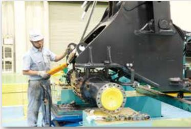
After the frame is assembled on the frame assembly sub-line, the axles and fuel tank are attached. Then the front frame and rear frame are joined.
