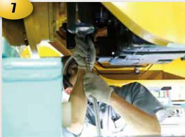
The drive shaft is attached. Workers enter the work pit and perform work operations from beneath the equipment body.
