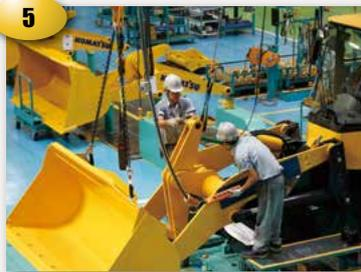
The boom and bucket are attached. A dramatic increase in productivity is achieved by transporting the boom and bucket with cranes set at different height levels. Previously, this process was handled by one large crane.
