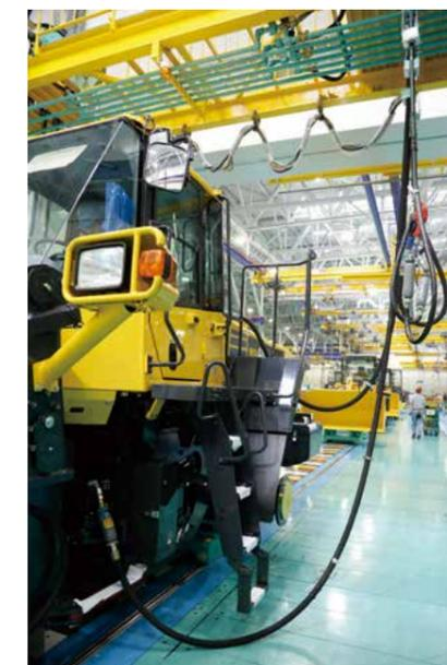
To accurately respond to complex orders, the hose for the particular type of fuel automatically descends from above by calling up data.
