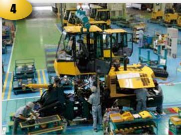
The cabin is mounted on the frame.
