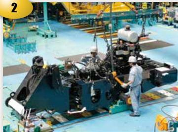
The engine is fitted and engine unit pipework is performed.
