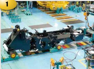
The frame is set onto the main production line. A conveyor pulls the main line forward at a speed of 50 cm (20 in) per minute. A counterweight is mounted.
