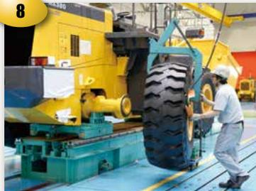
The tires are fitted. Two cranes and a specialized hoisting machine lift the tires to the wheel hubs and the wheel nuts are tightened with a specialized nut runner.
