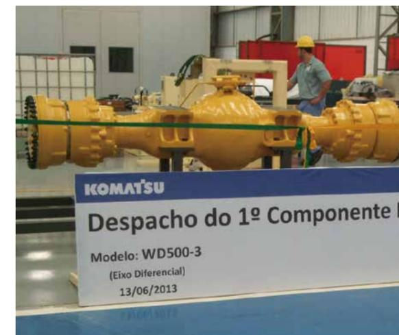
Remanufactured axle for WD500 wheel dozers at Reman center, KDB
