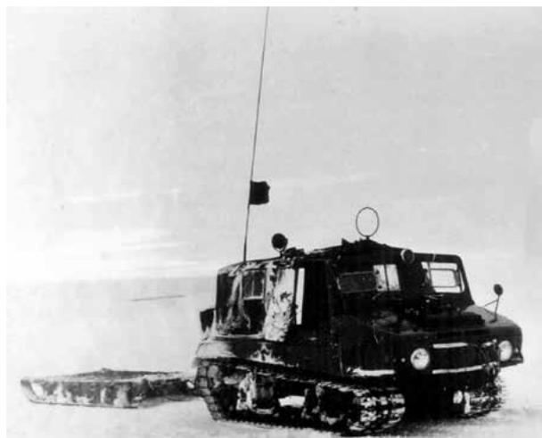
KC20, a Komatsu snow vehicle manufactured in the 1950s and delivered to work in Antarctica (Komatsu no longer manufactures snow vehicles.)
