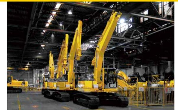
Inspection line for hydraulic excavators
