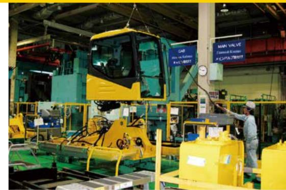
Mounting an operator's cabin on a medium-size hydraulic excavator
