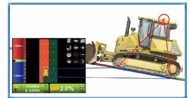
With the data collected by the cab-top GNSS antenna, the height of the ground surface where the crawler track is in contact is computed and displayed on the monitor.
